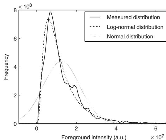
**Fig. 3.** Measured distribution of foreground intensities agrees with lognormal distribution. Its asymmetry is in contradiction with normal distribution.
