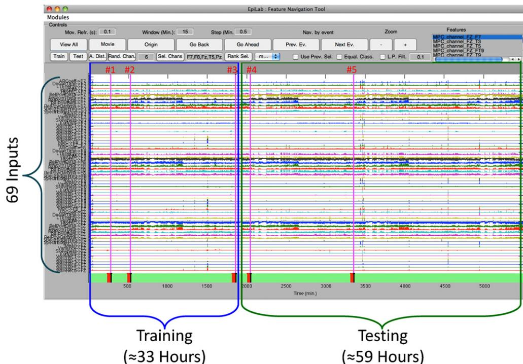
**Fig. 8.** Feature navigation window with the input dataset and respective training/testing division. The vertical black lines represent the different seizures onset epoch (#1, ..., #5).
