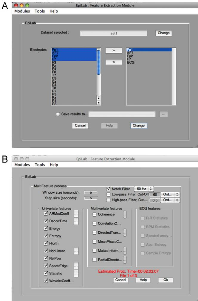
**Fig. 3.** Feature extraction windows: (A) Window that enables the selection of the electrodes to be involved in the feature extraction procedure. (B) Window that enables the selection of the feature to be computed, as well as the window and step size used for the features computation.
