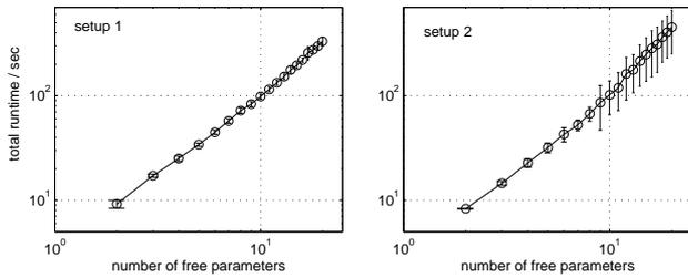
**Fig. 2.** Dependency of the total runtime on the number of free parameters, plotted double logarithmically. The exponent of the non-linearity is  $\approx 1.56$  for setup 1 (left panel) and  $\approx 1.78$  for setup 2 (right panel). Error bars reflect variability within the set of free parameters.
