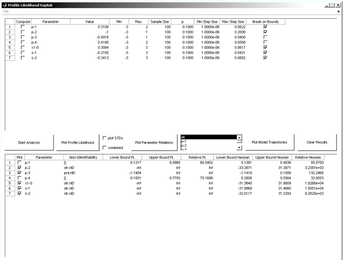
Fig. 3. The Graphical User Interface. The upper table contains information about the parameters and allows to specify tuning values for the algorithm. All necessary function calls can be accessed via buttons in the center. The lower table displays the results of the analysis. All values are given in orders of magnitude using  $\log_{10}$ .
