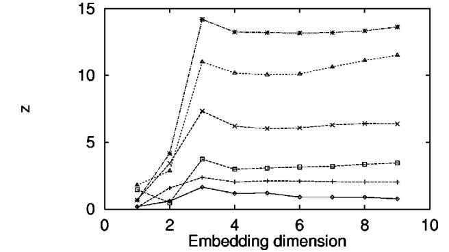
FIG. 3. Results of the simulation study for the amplitude modulated process. Shown is  $z$  in dependence on the embedding dimension for different degrees  $M_{\text{amp}}$  of violation ( $\diamond = 0$ ,  $+$  = 0.1,  $\square$  = 0.2,  $\times$  = 0.3,  $\triangle$  = 0.4,  $*$  = 0.5).
